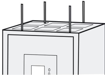
Install the spacers. The longer spacers must be positioned toward the front of the UPS.
