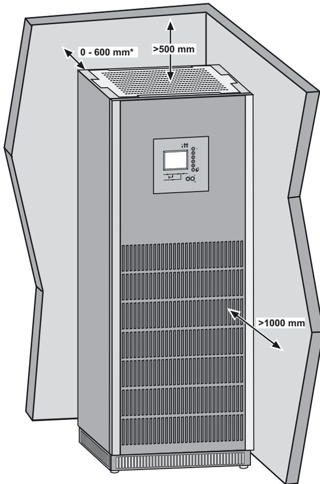
To ensure correct ventilation, leave nothing on top of the UPS.
