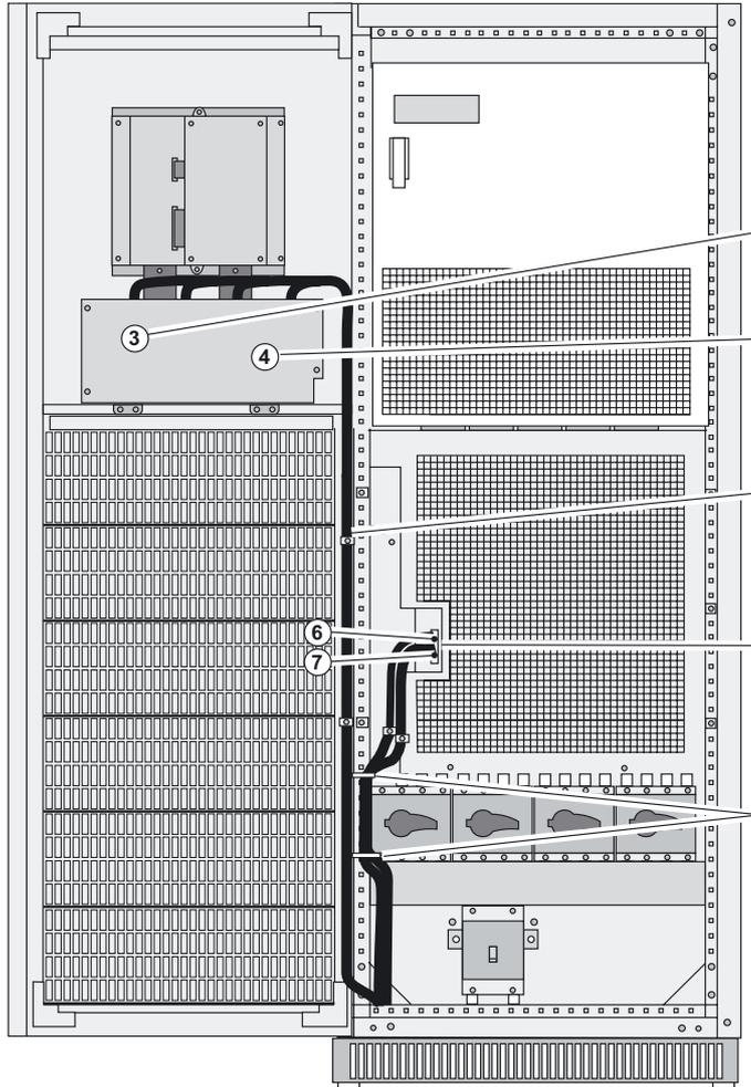
Separate the control and communication cables from the power cables.
