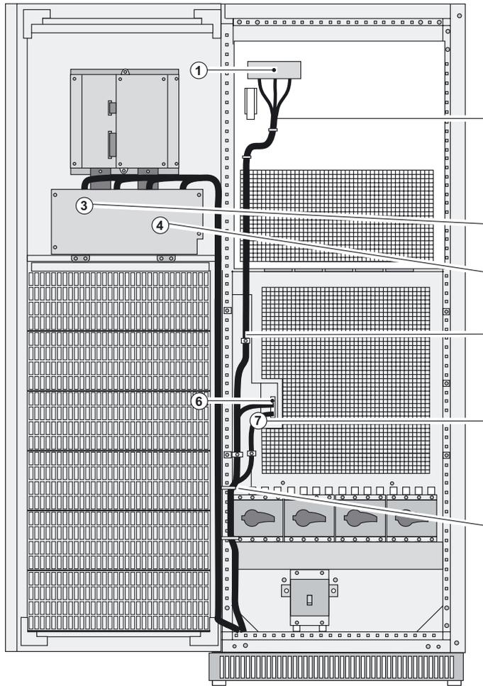
Parallel-connection cables for connection to the external bypass cabinet (not supplied max. 2.5 mm<sup>2</sup>). The CAN and I exchange cables are supplied.
