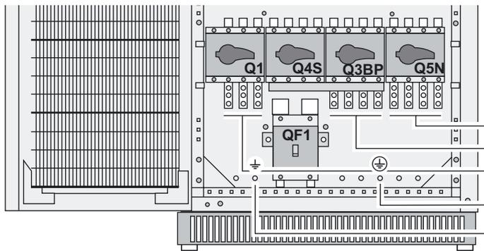
View with terminal-block protection cover removed
