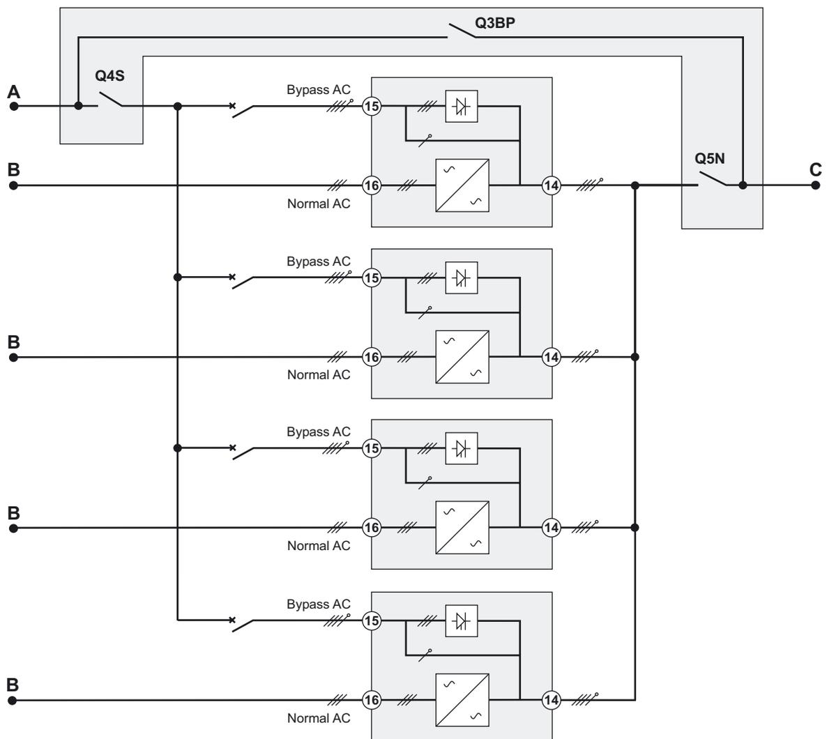
Connection for the Bypass AC input and the output cables to the external bypass cabinet must use cables having the same length and size to ensure correct balancing of the Bypass AC input currents.
