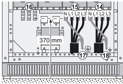
1. Connect the power network cable PEN to the UPS earthing terminal
